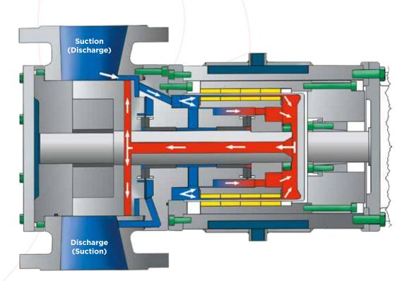
One of the distinguished features of the ROTAN® ED range is that the pumped medium is hermetically contained in the system since the magnetic coupling eliminates the need for a shaft and mechanical seal, which could allow gaseous exchange between the pumped medium and the atmosphere.
